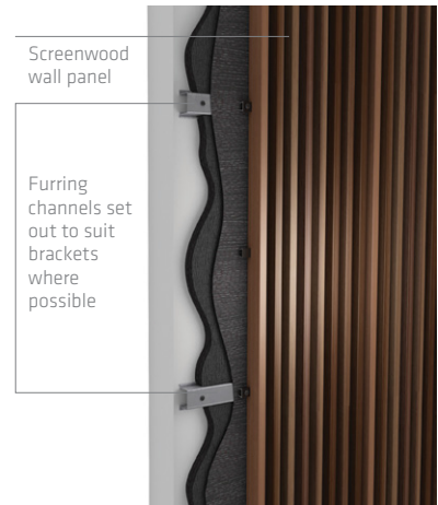
Detail: Section through vertical wall application with SC15 acoustic scrim and SCP50 batts
